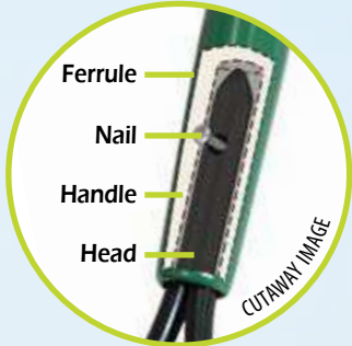
Nail is driven through ferrule, handle, and rake head
