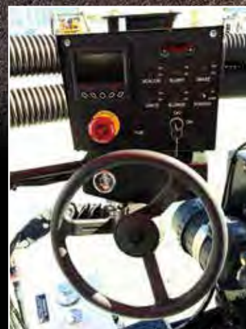
Digital Engine Panel, Fuel Gauge and E-Stop
