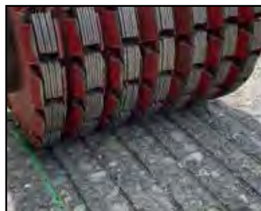
MILLING DRUM WITH PCD PLATES
