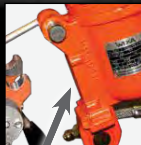
Integrated motor mount for Weka DK22F and DK32F only
