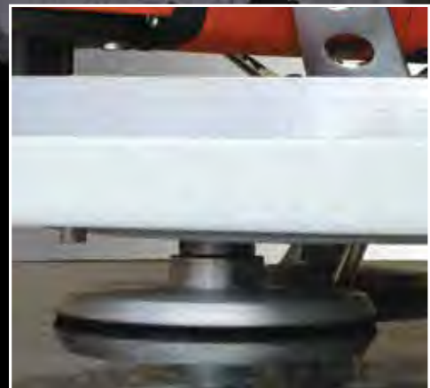
One of three 5" grinding platens (Velcro® surface)
