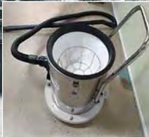
Pre-Filter for Dry Containment
