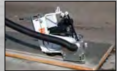
CC190PRO-EE with CVG1-PRO hose attached to side vacuum plate
