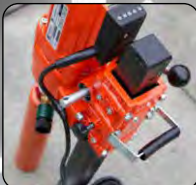
Built-in LED Light Amp Meter
