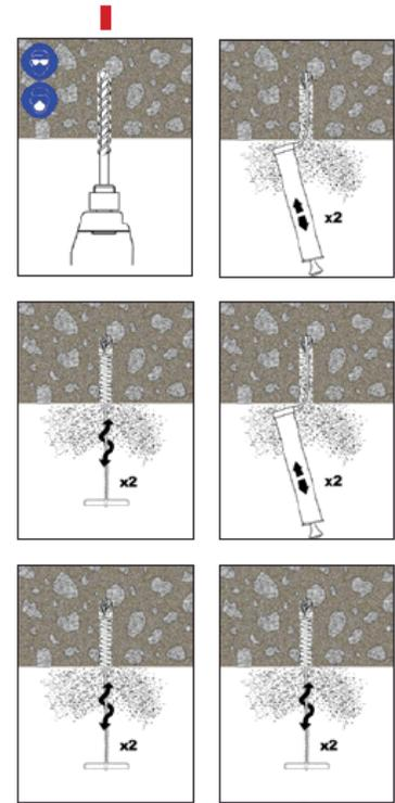
hole collects water after the initial cleaning, this must be removed before injecting the resin.
