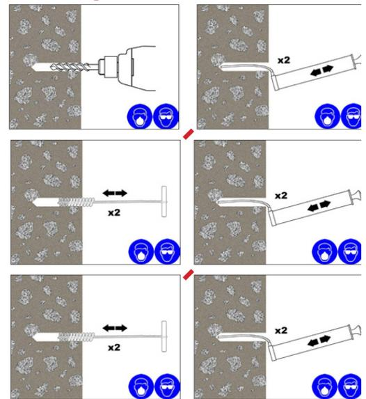
*If the hole collects water after the initial cleaning, this water must be removed before injecting the resin.*
