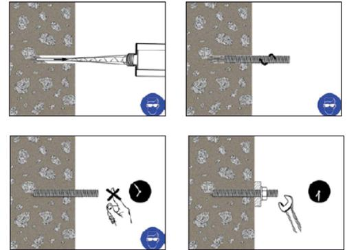
**Note for decreased installation temperature:** When installing EASF at decreased installation temperature (+32°F < T < 50°F (0°C < T < +10°C)) the cartridge must be conditioned to +68°F (+20°C)
