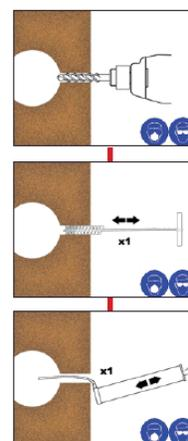
*If the hole collects water after the initial cleaning, this water must be removed before injecting the resin.*
