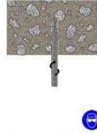
12. Clean any excess resin from around the mouth of the hole.
