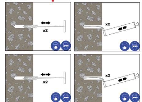
If the hole collects water after the initial cleaning, this water must be removed before injecting the resin.
