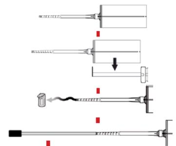
free from oil or other release agents. Insert the steel element to the bottom of the hole using a back and forth twisting motion. Any excess resin should be expelled from the hole evenly around the steel element.
