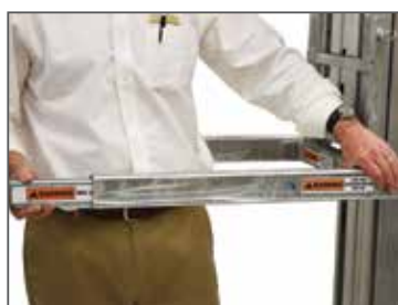
With push of a button, optional fork extensions extend forks extra 8" / 20 cm. Extensions store in forks. Extension capacity 450lb / 205kg. Part # 783163.
