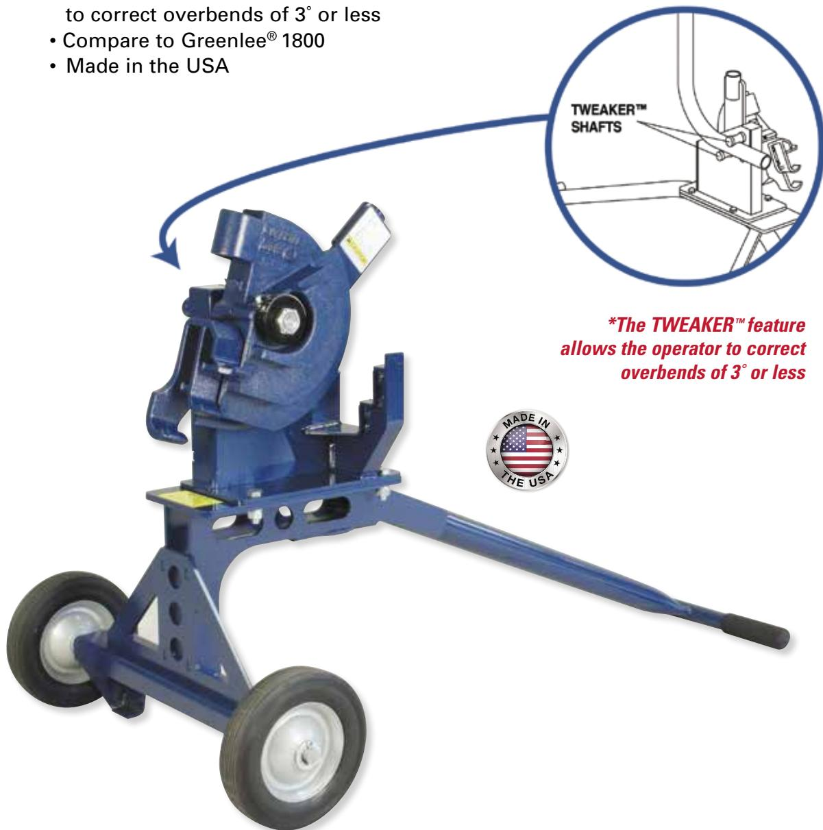
*\*The TWEAKER™ feature allows the operator to correct overbends of 3° or less*
